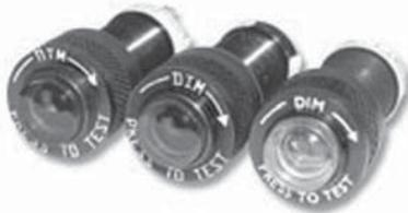
Miniature press-to-test indicator with built-in bulb testing device. Adjustable dimmer. Uses #330 (12V) or #327 (24V) bulb. Bulbs NOT included, order separately.
