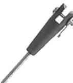
**RC8-7 CLEVIS/PUSHROD KIT** - Contains two 8-32 threaded clevis forks; 7" long, 8-32 threaded, stainless steel pushrod and hardware. This kit included with Ray Allen trim systems. NOT compatible with POS series position sensors. The T4-5 clevis/pushrod kit has just one clevis assembly. RC8 clevis & its hardware are available separately. RC8-7 Kit ..... P/N 11-02040
