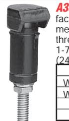
**A350 WHELEN POST LIGHTS** - For illuminating instrument face. The 1" long 8-32 threaded shank serves as instrument mounting screw. Terminal on end of shank mates with threaded connector on insulated wire lead. Overall length 1-7/8". Blue tinted filter or red filter. With #330 (12V) or #327 (24V) bulb. Order by Part No. ALL
