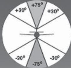
An approved anti-collision strobe light system must project light + or - 30° above and below the horizontal plane of the aircraft. One or more strobe lights can be used. The + or - 75° projected light is required since July 18, 1977.
