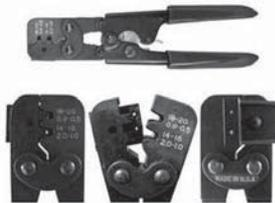
Crimps Seal-All terminals and seals in one cycle. Features two double Cavities, an orientation block and a ratchet mechanism to ensure that each crimp cycle is completed. Factory calibrated to be used only with Seal-All terminals and seals. Wire range 20-14.
