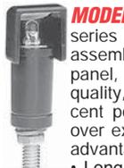
**MODEL 70844 SERIES LED POST LIGHTS** - The model 70844 series are LED (Light Emitting Diode) instrument post light assemblies. They are designed to illuminate the instrument panel, and function as instrument mounting bolts. It is a high quality, long lasting, modern alternative to standard incandescent post lights. They offer significant technological upgrades over existing products. Utilizing LED technology, the following advantages are offered:
