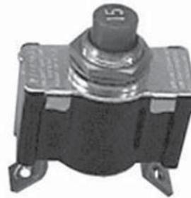
Feature a bi-metallic snap-acting disc as the sensing element. Widely used in production and military aircraft. The most popular models are illustrated. Models PSM and PSM-N are available in the following ampere ratings: 2, 3, 5, 10, 15, 20, 25, 35. When ordering specify if neck-mounting style is wanted by placing "N" after ampere rating. Example: PSM-10N (P/N 11-04244)..... Ea.
