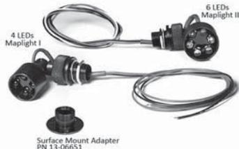
The body of the maplight is constructed of aircraft grade 6061 T6 aluminum and black anodize treated for protection from corrosion. The LED bulbs and internal components are high quality components, and are engineered to withstand 150% of their rated voltage without damage. The wire is
