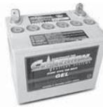
•Maintenance-free operation •Excellent shelf life •Long cycle life •Can be mounted on its side •Delivered fully charged and ready for use •Quality construction provides superior resistance to shock and vibration •Long life w/a charging voltage of 13.8V +/- .2V •Need adjustable voltage regulator such as the LR-3 so that charging voltage can be set at 13.8V •No corrosive gas generation •DOT & IATA approved for shipment by air as dry cells •300 Starting AMPS •Warranty 1 year or 100 hours.
