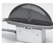
**MODEL 90033 SERIES SELF-CONTAINED LIGHT ASSEMBLIES** - 90033 series self-contained, 150 watt, quartz halogen flashing anti-collision light which is factory installed on Beechcraft. It is also a direct replacement for oscillating beacons on most corporate aircraft.
