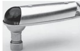
**MODEL A675 SERIES** - A675 series wing tip position and taillight designed to eliminate the need for a tail mounted position light. It uses a 26 watt incandescent lamp for the forward position light and a 25 watt halogen for the tail position light. Specify 14 or 28 VDC.
