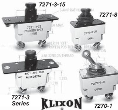
The Klixon 7270/7271 series circuit breakers were designed to utilize less behind panel space while protecting wire and cable in aircraft and ground support equipment on either 120 VAC, 400 Hz or 30 VDC systems. The units are available with neck mounting (7270-1 and 7271-8) or standard cover plate (7270-7 and 7271-3). In each of these Klixon circuit breakers, the bi-metallic element assures uniform current distribution throughout
