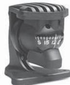
Navigator NV2-2400 by SIRS is designed to replace older, less stable compasses. The NV2-2400 bolts onto the aircraft's glareshield. The Navigator houses a compass rose suspended in a silicone-based fluid and features silicone seals to eliminate the problem of leaks and fluid evaporation common to older compasses and reduces lead and lag errors inherent in liquid-filled compasses. Metal expansion bellows allow
