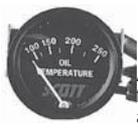
A quality gauge which is complete with all installation fittings. Range is 100 -250 F. 5/16-18 female capillary adapter fitting. 60" lead length.
