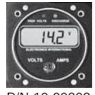
**VOLTS/AMPS - VA-1A, VOLTS/AMP.** STCd, PMAd as PRIMAR REPLACEMENT. Internal Shunt. Discharge High Voltage Warning Lights. 100 amp capability. .1 volt & .1 amp 1% Resolution. Accuracy: 2 1/4" Mount. 2.5" Depth. 9 Oz. Unit. Viewable in direct sunlight. Backlit. Operates from 7.0 to 40 volts .1 amp.
