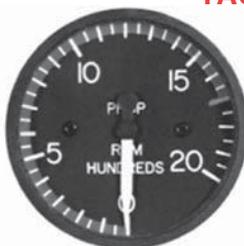
2" Prop Tachometer, Green Arc from 0 RPM to Red Line at 1700 RPM
