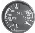
High accuracy 2" pressure gauge that qualifies per mil-g-7734c, and has standard wet-line connection. Oil temperature is sensed by a MS28034-1 resistance bulb. Dimensions: 2-3/8" 2-3/8" 2 Weight: .5 lbs. Power: 0 to 200 PSI & 0-300 PSI.....P/N 10-02075
