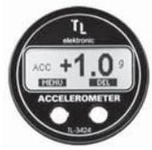
The TL-3424 is complete weight acceleration management. The instrument incorporates a high-precision sensor for measuring acceleration in the vertical axis. The SAS version also incorporates a sensor for measuring the indicated airspeed, which enables the activation of memory recording. Both versions enable to utilize an undercarriage scanner that can also activate memory recording.
