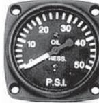
These factory new oil pressure gauges from UMA fit standard 2-1/4" panel hole. They are mechanical, wet-line gauges and require no sending unit.
