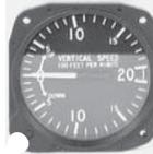
The vertical speed indicator is a precision instrument which provides an accurate indication of rate of change of altitude. This instrument is temperature compensated and is provided with a zero adjustment screw on the face of the case in the seven o'clock position. Power: Static system.
