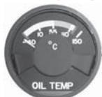
Housed in a 2" diameter case, this top quality Kelly Manufacturing Co. oil temperature gauge is operated by an MS28034-1 resistance bulb and is available in C or F scale. Size: 2" dia. x 3.12" long. Wt. 4lbs Power: 28VDC Connector: MS3112E8-4P. Add -C or -F to part no. for C or F.
