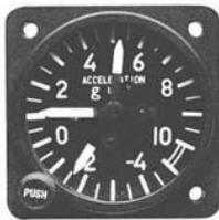
Accelerometers register to "g" forces acting on the airframe during turbulence or aerobatic maneuvers. One pointer gives a continuous reading, the other two indicate maximum positive and negative loads. Easy to reset by pushing the "push to reset" knob.
