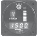
Available in 4 or 6 cylinder configurations • Supports most type K thermocouple probes • Displays information in C & F with automatic conversion of all setup parameters • Accuracy to within 1°F • Displays temps from 0 F – 1900 C / 0 C 1040 C (EGT) 0 F – 700 C / 0°C – 371°C (CHT) • High speed scan and acquisition rates. While others update information every 5 seconds
