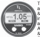
TL-3624 is suitable for most aircraft whether they be airplanes or whether they be gliders. • Measure climb & descent rate with high level of accuracy using the integrated or averaging memory with selectable averaging time • Set value limits at 2 levels (Warning & Alarm) for climb and descent rate • Use acoustic climb & descent rate signals using an external loudspeaker. Size: 2-1/4"
