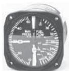
This space saving 3-1/8" gauge provides manifold pressure (10"-50" Hg) and fuel flow (4-36 GPH). New manufacture by United Instruments. Direct connections. No transducer required.....P/N 10-10200
