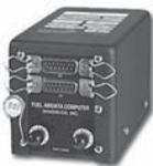
The affordable Shadin F/ADC-200 Fuel/Air data computer maximizes aircraft range and fuel economy by providing automatic updating to your GPS for true air speed, winds aloft, wind components, density altitude, OAT, pressure altitude, fuel flow rate, fuel used, fuel required to destination, fuel endurance, and more. Interfaces with most popular GPS units including Bendix King KLN series, Garmin 150, 155, 165, Trimble
