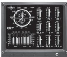
True TFT Transflective Custom Display - Display brightness increases with ambient brightness, always sunlight readable. All gages have a Variable Scale and alarm limit to fit your engine. New form factor, panel size: 6" w 4" h 2.9" d. Records all engine parameters at 2 to 255 second intervals. Plot the data with E plot. All probes and transducers supplied. High Flow transducer (120 GPH) included in EDM930T. Compatible with and transmits RS-232 data to most MFD's, also sold less the display.
