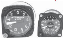
This instrument registers "G" forces acting on the airframe during turbulence or aerobatic maneuvers. One pointer gives a continuous reading, the other 2 indicate maximum positive & negative loads. A reset knob is provided. In smooth, level flight the instrument indicates +1 "G". Large "G" Meter - Range: -5G to +12G.
