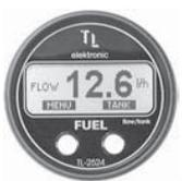
• Measure immediate fuel flow of your engine in liters/hour or liters/100 km and average fuel consumption • Set limit values at 2 levels (Warning & Alarm), for all measured values. In case these values are exceeded, the instrument will warn you prior possible failure or damage of the engine • Display at any time the fuel levels in the left, right or both fuel tanks. Size: 2-1/4"
