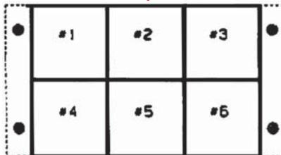
Available in 6 gauge (pictured) or 8 gauge clusters. On 8 gauge clusters, 2 additional gauges are added to the right side of the one pictured. Specify gauge and position desired for all cluster gauge positions. Prices are for the backplane (panel) only. Add price of
