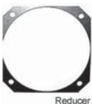
**3ATI Reducers to 3 1/8"** - Use a 3ATI hole cut out to mount 3 1/8" diameter instrument. Plate can be shimmed to instrument panel thickness. Simple installation. Heat-treated aluminum .080 thick with black anodize finish. P/N 07-01331 .....
