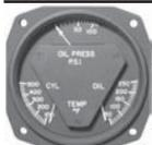
**18-1002 SERIES** - This gage consists of three moving coil meter movements within a 3" diameter case. Oil temperature is sensed by an MS28034-1 resistance bulb and cylinder head temperature is sensed by an AN5546-1 resistance bulb. Oil pressure is sensed by a VDO Transducer. Connection is made by a single cannon type connector: Part Number MS3106A-14S-6S.
