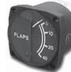
This 2-1/4" flap indicator uses a resistance potentiometer as a flap position sensor. Transmitter required. Wt: 9.8 oz.
