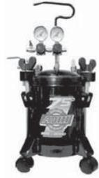
**65-911** - 2-1/2 gal. pressure tank, single regulator, Teflon coated inside and outside Safety relief valve, pick-up tube with filter, wide lid and low side walls, large wheels for easy movement. P/N 12-02117 .....
