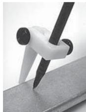
This handy device holds a marking pen and has an adjustable stop for running along the edge of a part. The adjustable stop allows variable edge distance for rivet layout, etc. One thumbscrew holds the pen (pen sold separately) and the other thumbscrew holds the adjustable stop. Made from delrin (plastic) material. Comes ready to use with (1) Pilot marking pen. P/N 12-00630
