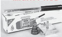
Designed to bend solid round, square and flat alloys into nearly any shape and angle. FEATURES: • Works on solid materials up to 3/8" diameter. • Coils and bends wires of many sizes. • Includes dies for 1/2", 3/4", 1", 1 1/4" & 1-1/2" diameter bends. • Constructed of 3" x 3" aluminum base 1" thick with a 12" handle 7/8" in diameter. • Made in the USA. • 1 year Replacement Warranty. P/N 12-00934 .....
