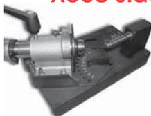
Constructed of 6061T6 hard anodized aluminum extrusions, steel, and cast iron with two 2750 lb. rated roller needle bearings, the Accu-Jigger rigidly holds the holesaw and tube to produce accurate, chatterless cuts. Accu-Jigger, with Single Point Technology, is able to notch tubes that "Fit Right The First Time" as fast as those produced from custom tooling. It
