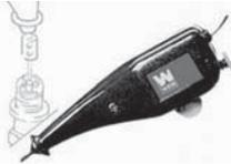
Anyone that cleans a lot of spark plugs knows that a spark plug vibrator cleaner is the only way to go to break up and clean
