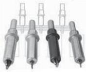
**K-SERIES SPRING CLECOS** - Sheet holders provide the quickest method for holding sheets together for drilling or riveting. Drill the size hole needed for the rivet and insert the sheet holder. The holders listed comprise the most common sizes. Material thickness range 0" - 1/4". Use with sheet holder pliers. **10% discount on 50 pcs.,**
