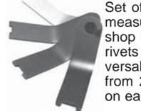
Set of four gauges for -3, -4, -5, -6 rivets. Each gauge measures Minimum height and Minimum diameter of shop heads AFTER setting. Eliminates guessing if your rivets are properly set. Works for measuring both universal head and flush rivets. Precision machined to size from 2024 aluminum. Rivet size permanently stamped on each gauge. Color coded anodized finish. P/N 12-01533
