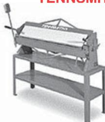
**HAND BRAKE & STAND** - Versatile, economical hand brake designed for straight forming of mild steel in thicknesses of 22 gauge & lighter. Made in the U.S.A by Tennsmith. Bends material up to 48" wide. Wts: brake: 280 lbs. Optional stand: 95 lbs. Ideal for bending materials used in light aircraft construction. Shipped direct to you from factory in Tennessee.
