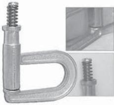
Spring tension clamps can be applied in a fraction of the time required for ordinary screw clamps. The AT542 clamp, with 2" throat depth, has a Zamak alloy yoke and a steel spring which provides a 70 lb. clamping pressure. Designed for use with sheet holder pliers.
