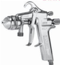
The Binks Mach 1 HVLP is a siphon-fed refinishing system that performs like your favorite conventional outfit but produces far superior transfer efficiency. A unique arrangement of air nozzle, fluid nozzle, and needle enable the Mach 1 to draw material from a standard siphon feed cup and avoid the need for a pressure cup. Eliminates the need for the operator to set fluid pressures. Delivers lower emissions for compliance with environmental regulations.
