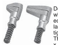
Designed to hold two or more work pieces together where no holes exist. Clamping force is applied at edge of work. Spring loaded, plier actuated. The lack of a takeup screw makes it impossible to over-tighten and damage the work surfaces or the clamp. There are 4 standard sizes : 1/2 x 1/2", 1/2 x 1", 3/4 x 1/2", 3/4 x 1".
