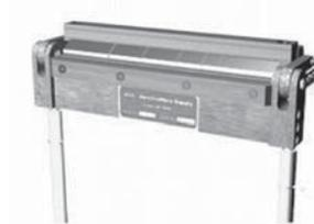
This small, compact brake is excellent for all tough fabrication and repair jobs. The radiused dies make it possible to form those difficult materials such as 2024T3, 4130, and stainless without fear of cracks. Features solid steel bar construction, heavy duty clevis hinges, and portable bench mounting. Includes 2 sets of assorted width reversible dies with 1/16", 1/18", and 3/16" radii, plus complete
