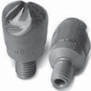
Designed for operating in angle drills with 1/4-28 threads and in the AT441SLS Micro Stop Countersink. Has 1/4-28 threaded shank. Cutter angle 100°. AT455D-4 has 7/16" dia. cutter head. Use with AT484 pilots. P/N AT455D-4.....
