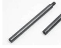
Use these different length extensions in your 90° or 45° drills. 1/4"-28 male threads on one end and 1/4"-28 female threads on other. Comes in three different lengths 1" 2" 4". 2" ..... P/N 12-01541
