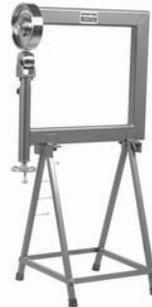
Clearly, this is the most popular of in-home English Wheels. Trick out your custom-built bike or complete hobby projects without breaking the bank. Provides outstanding performance on small jobs like motorcycle tanks, tank covers, seat cowls and aircraft fillets. Versatile use - mount on bench, clamp in vise or use with optional welded stand.
