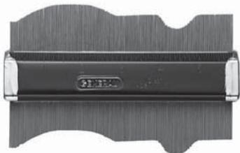
General's 6" Contour Gage is designed for precise surface duplication in woodworking, fine carpentry and other professional genres. The 35 ultra-thin leaves per inch assure that you are getting an exact replication of your copied shape. The Contour Gage is capable of duplicating surfaces up to 3-1/2" deep. Instructions: 1. Press Contour Gage against surface
