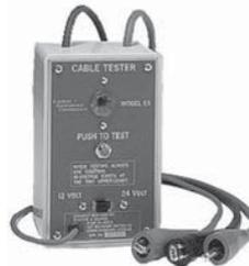
Gives a fast, accurate test of high voltage aircraft ignition cables. Simply connect 3 wires, push test button and test is completed. The E5 will instantly indicate in its test window both good and defective cables - no waiting for indication to appear. Fail-safe circuitry. Heavy-duty lead wires. Compact 3" x 5" x 2-5/8" case. Wt. 1-1/2 lbs. P/N 12-01016.....
