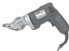
**ELECTRIC MODEL K-200** – Extra-powerful 115V, 50/60 cycle AC/DC motor. Heavy-duty bearings & die-cast aluminum cutting head. Tool is UL and CSA approved. 2300rpm. Maximum cutting speed, 180 inches/minute. Wt. 5 lbs. Over-all length, 11.75". Ampere rating, 2.2 amps. P/N 12-01137.....
