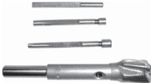
The Spotface It tool makes a flat spot for screws. This tool is specifically modified to provide rail cap clearance for use on seat rails. Cutter comes with 1/8, 5/32, 3/16 pilots. P/N 05-04429
