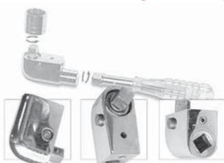
This tool is a combination tool providing a ratchet wrench for power and a spinning action for speed. All types of accessories can be used with this wrench, such as extensions on either end, or flexible drives. The drive handle can be removed to make a very compact tool for restricted areas. The ratchet pawl is made from annealed steel to allow it to fail before the ratchet
