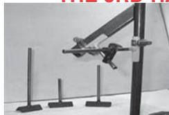
A simple yet rugged tool, The 3rd Hand was designed to hold round or square tubing in place during the welding process. Originally used for aircraft engine mount and airframe fabrication work, it has many other applications. This steel fixture is infinitely adjustable due to its full swiveling clamp. Each model comes with 3 different length arms (3.5",
