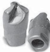
Three-straight flute replaceable pilot cutters with female thread. These cutters are designed with extra deep flute to permit numerous sharpenings and radial clearance to assure fast smooth cutting.
