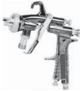
**6008SSPXX** - HVLP Water Base Spray gun, die cast aluminum body, low cfm [4-6], SS fluid passages. replace xx with 1.0, 1.3, 1.4, 1.5, 1.8, 2.0, 2.5 for tip size P/N 12-02136.....
