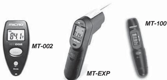
Digital, non-contact infrared thermometers are used for hundreds of practical applications and are essential tools for professional automotive and aviation technicians.
