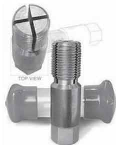
In servicing spark plugs, a common problem is carbon accumulation in the jug threads. Cleaning these threads regularly can save big money by preventing thread damage and the need to pull the jug and install thread inserts. This specially designed tool works very well to limit this problem. It provides maximum depth penetration and its unique spring action assures that there will be no enlargement of the existing thread pitch diameter. P/N 12-17200 .....
