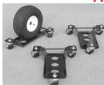
AeroRoller makes movement of your aircraft or wheeled equipment easy. Aircraft can be loaded on AeroRoller without jack and minimum effort is required to move aircraft when on rollers. AeroRoller is constructed of Industrial 1/4" steel plate. Heavy duty Duraform 360° swivel castor wheels means no flat spots. Brake castor lock parking location. Each unit can carry 1000 lbs.
