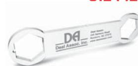
The 1" hexes of the wrench easily fit Champion oil filters. The hexes are rotated 15 degrees from each other so by turning the wrench over or flipping it end-for-end you can easily find an orientation that allows you to get on the filter, even the tightest engine compartment. It's 6 inch overall length allows you to turn it tight locations, and the shorter length helps prevent over-tightening the filter during installation. P/N 12-01638 .....
