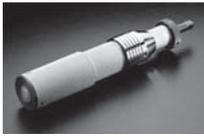
The MD1F35H is an adjustable driver with a range of 5 to 35 lb. in. Body is constructed of steel and anodize aluminum, has a CNC machined knurled grip and 1/4" male drive and comes packaged in a plastic box. The MDP1F35 is a preset model ideal for repetitive assembly operations. P/N 12-00530
