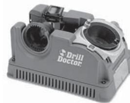
The DD500X Pro Kit combines the Drill Doctor Tradesman sharpener with heavy duty carrying case. Sharpens bits either 118° or the high performance 135° setting and it can turn standard drill bits into self-centering, split point bits. Sharpens bits from 3/32" to 1/2" diameter in about
