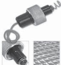
The timing jumpers are easily used for timing magnetos without removing the breaker box cover. Simply remove the "P" lead and replace with timing jumper. Then hook up timing light leads. These handy devices have proven to be a real time saver and, in some cases, an outright necessity. **SOLD IN PAIRS**
