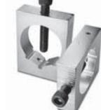
Designed to enable safety wire holes to be drilled through the head of bolts or through nuts, across the diagonal. Designed to accept up to 3/4" dia. nut. Easy to use. Nut Saf-T-Blok requires that the nut or bolt be placed into the "V" groove, tighten down the holding screw, drill & deburr.
