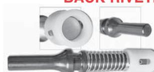
For back riveting flush rivets on RV control surfaces and other home-buils. Has a plastic Delrin sleeve with spring to hold multiple sheets of aluminum together while riveting. 0.401 shank x 4-1/8 inches long.
