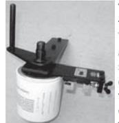
This tool was designed to eliminate much of the mess that occurs with small handheld oil filter cutting tools. Very simple to operate, it is excellent for individual aircraft owners as well as FBO's and maintenance shops where a lot of filters need to be cut. Simply clamp in a vise, screw on the filter, turn the cutter into the filter and hand crank to open the filter. The rugged construction enables this tool to operate trouble free for years.
