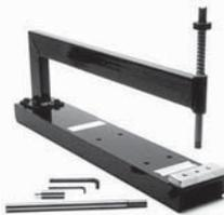
Features include: • 22" deep x 4" tall throat • Heavy wall 1" x 2" steel tube arm • Heavy wall aluminum channel base • Bronze 1/2" I.D. guide bushings for shafts • Heat treated and
