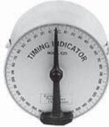
This all-aluminum unit improves and speeds up the timing of magnetos to the engine. Easily attached to propeller spinner, it is accurate to within 1/2 degree. Has easy to read dial and comes with top dead center locator and mounting bands. P/N 12-01014.....
