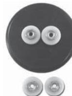
For pre-bending skin edges on lap joints and butt joints before riveting. "Edge rolling" will prevent skin edges from curling up during riveting. Machined round body made from 2024 aluminum. Hard black anodized finish for wear resistance. Ball bearing style nylon rollers (non marking); + spare set of rollers and instructions included. P/N 12-00632
