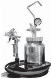
**RP-XX** - 2 Qt. pressure pot outfit includes an R100 mini gun, 2 qt. pressure pot with regulator and 6' air and fluid hose with fittings. This outfit is especially designed to spray in hard to reach areas. Suitable for both water and solvent base material.
