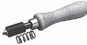
Slotted type cowling fasteners are not easy to fit with generic common screwdrivers. To overcome this, driver has a broad hollow cut tip that accurately engages the drive slot. Additionally, a no mar, spring loaded, plastic sleeve simultaneously guides the tip by fitting around the outside diameter of the fastener head. P/N 12-17615.....
