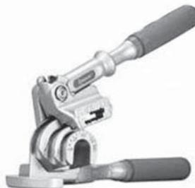
The 470-FH Triple Head 180° Tube Bender bends 4 diameters of tubing with just one tool! It handles soft copper, aluminum and thin-walled steel tubing in 3/16", 1/4", 5/16" & 3/8" diameters. Like the heavy duty 464-FH, it features the patented ROTO-LOK™ two-stage handle that allows east fabrication of bends up to 180°. It also features optimized bending grooves that allow the user to bend the tubing in the smallest
