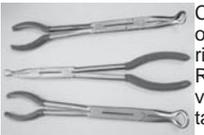
Compound joint allows access in long narrow openings with minimal handle movement. Flush-riveted joints contribute to the tool's narrow profile. Red vinyl grips for comfort & control. Chrome vanadium material for durability & corrosion resistance. 8mm Pliers .....P/N 12-01344
