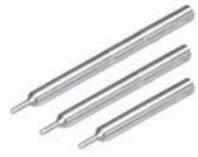
Use these different length extensions in your 90° or 45° drills. 1/4"-28 male threads on one end and 1/4"-28 female threads on other. 2" ..... P/N 12-01535
