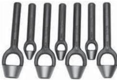
Our extensive selection of Arch Punches are machined to close tolerances for creating precise holes in gasket material, rubber and soft metals. These industrial-quality tools are hand forged to ensure the longevity and accuracy of the cutting edge. This seven-piece set includes some of our most popular punch sizes and is conveniently packaged
