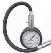
This very accurate bourdon tube tire gauge offers precision pressure control and a rugged steel case with rubber shock-absorbing cover. It comes complete with a 12" long flexible braided hose, a bleeder valve, and stop hand. It is easy to read the pressure on this 2" gauge with 1" psi markings and 60 lb. range. Excellent for use on aircraft tires as well as cars and trucks.
