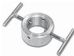
Precise Gap is a simple tool to gap two-, three- or four electrode 18 mm sparkplugs. Only 2" overall - comfortably handheld. Precision made of stainless steel. "T" handle adjusters move the ground electrodes closer to the center electrode until wire feeler identifies proper gap. Adjusters have
