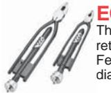
These top quality twisting lock pliers with automatic return are economically priced and extremely durable. Features a sharp cutting edge and will twist up to .060" dia. safety wire. Length 6" & 9". Foreign made. 6" ..... P/N 12-01472
