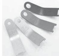
Set of four gauges for -3, -4, -5, & -6 rivets. Each gauge measures MINIMUM height and MINIMUM diameter of shop heads AFTER setting. Eliminates guessing if your rivets are properly set. Works for measuring both universal head and flush rivets. Precision machined to size from 2024 aluminum. Rivet size permanently stamped on each gauge. Color coded anodized finish. Instructions included. P/N 12-00631
