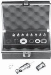
This kit provides countersinking versatility with nine different 1/2" diameter cutters, six of the most commonly used foot pieces, and a high-speed bearing-constructed microstop. The microstop controls cutting depth in .001 increments, from 0 to 5/16". Cutters-ground on-centers to ensure concentricity-are 100°, with pilot diameters #40, #30, #21, 3/32", 1/8", 3/16", and 1/4".
