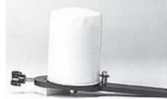
This aviation oil filter cutter will open any size oil filter canisters for your inspection. To use the tool, place the filter in a vice, attach the tool to the top of the filter, and rotate 4 to 6 turns to open the canister. The cutting wheel will stay sharp for about 50 uses, and is easily replaced when dull.
