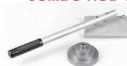
Constructed of 4" x 6" aluminum base 1" thick with a 16" handle 7/8" diameter. Bends solid round, square and flat iron. FEATURES: • Works on solid materials of up to 3/8" round and square (1/2" wide flat). • Coils and bends wire of many sizes. • Bends metal to any shape and degree of angle. • Include dies for 3/8", 3/4", 2", 3" & 4" diameter bends. • Installs on any vise. • Ideal for hobbyists, prototype shops and do-it-yourselfers. • Made in the USA. P/N 12-00935 .....
