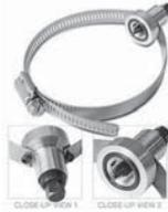
This oil filter drain tool permits draining spinon oil filter prior to removal from the engine. Just clamp on to rear of filter with cutter, punch small air bleed at the top of the housing with anice pick, remove cutter and oil will drain freely in-can or hose-extended funnel.
