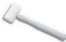
This custom made UHMW polyethylene plastic mallet is great for dimpling skins. Blows are more solid and much quieter than with steel hammers. Will outlast wood mallets. Hammer head measures 2.5" round x 4" long with 12" handle. Wt: 16oz. P/N 12-00605.....
