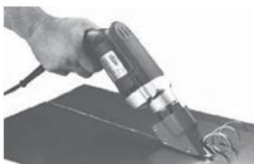
This lightweight, pistol grip shear cuts 14 gauge mild steel and most grades of stainless to 16 gauge. Double insulated, the KD 440 cuts over 150 inches/minute, leaving a clean, flat sheet, ready to fabricate. Distortions are absorbed in an easily disposed of waste curl, leaving the sheet cool and free of burn, chips, and burrs. The cutting blades are finest high speed steel. (Also cuts sheet metal, Stainless and Plastics) P/N 12-00676.....
