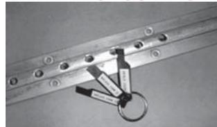
Allows for quick limit checking of seat rail hole and wear dimensions. Gage elements are made from heat treated blue tempered steel. Each element is marked to correspond to the limits set forth in the relevant ad. The three gage elements are linked together on a universal spiral key ring. P/N 12-01056.....
