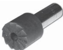
When substantial quantities of material have to be removed from the exhaust port, it may be necessary to also remove the island around the exhaust stud area. The ear island removal tool and pilot can be used to accomplish this without the use of power tools.
