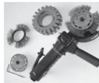
For the removal of seam sealant, corrosion, paint, vinyl decals, glue on aluminum and alloy.
