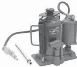
\* Designed for operating either manually or pneumatically \* Air hose can swivel in any direction \* Fitted with safety valve to prevent overloading \* Two piece handle allows for easy pumping \* Extension screw gives added height when necessary \* Minimum air pressure required is 90 PSI, 7 Bars \* Double spring return
