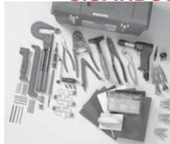
This kit is designed especially for the assembly of the Mustang Kit aircraft. It is comprised of over 300 items, specifically required in the fabrication and assembly of this aircraft.
