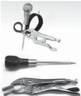
These special pliers allow for greatly simplified installation of single or multiple Adel type cushioned clamps. The pliers securely hold the aligned clamps in position, allowing for easy installation of securing hardware. Each kit includes special plier, alignment awl, and simple instructions. P/N 12-02017.....
