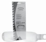
Each AOSAFETY Centurion® goggle TEAR-N-WEAR replacement lens protectors stack contains seven layers of high quality optically clear film. When the outer layer is soiled, scratched, or difficult to see through, simply "tear" the soiled layer off by pulling the tab horizontally from right to left. You now have clean and clear vision again and the next tab is automatically ready for your next tear away. P/N 12-00894 .....
