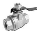
This J-3 fuel valve includes a steel handle for use with the original pushpull shut off control. This valve is a significant improvement over the original brass style fuel valve. The new valve has a stainless steel ball seated in an inert composite seat. This improved design eliminates the stiff operation and leaking around the shaft that the original design was prone to. PMA approved. P/N 05-00848
