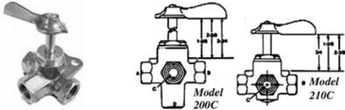
A full-flow plug valve with solid bottom and integral mounting bracket. Brass body and plug. Floating stem with O-ring prevents leakage. Packed with synthetic grease which resists gasoline and solvents. Indicating click on 3-port and 4-port valve (CN models) tells when handle is in full open or closed position. Tested to 30 PSI. Not FAA approved.
