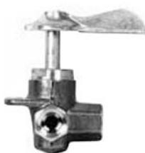
These 3-way Weatherhead valves, with 1/4" female pipe ports feature a Delrin-spool design for smooth operation. Handle mounted on 1-1/4" long shaft. Not FAA approved.
