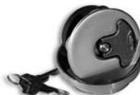
**GLASAIR FLUSH FITTING CAP** replaces the rubber seal Glasair cap (2.5-entry and 2" hole). Lockable. Epoxy/Flox in place. Based on aero 300 series. P/N 05-01004.....
