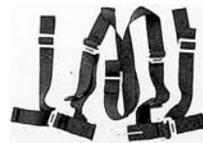
Complete pilot/passenger restraining systems for ultralights and experimentals. Made in the U.S.A., there's no stamped low-grade hardware in these top-quality sets. The webbing has a tensile strength of 6000 psi. These systems are designed for specific aircraft. Find yours in the
