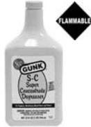
A concentrated self-emulsifying degreasing solvent for engine and parts. Dilute one part concentrate with nine parts of kerosine or light Diesel fuel oil for very effective cleaning. Spray or brush on. Does not harm electrical system, strip paint or cause rust. Water rinse.
