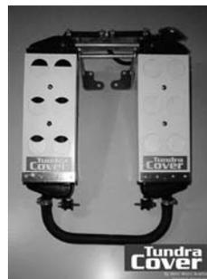
The Tundra Cover is designed to fit your Rotax radiators either from the front or rear. It is in-flight adjustable so you have complete control of your engines' temperature at all times.
