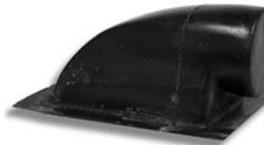
This lightweight air transition system provides the aircraft builder with an easy and simple way to supply cooling air to a firewall mounted oil cooler. Manufactured from composite materials, this duct system was designed to effectively and efficiently route cooling air to the oil cooler, thereby increasing the performance
