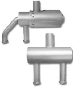
This universal stainless steel exhaust system is designed for experimental aircraft using Continental A65 thru O-200 engines. Consists of 2 manifolds, left hand manifold has heat shroud with 2-1/2" connection for carb heat. Muffler outlet are 3" long. Tailpipe extensions may be required, sold separately
