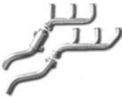
Fits Lycoming IO-540 (Angle Valve Engine) (Includes Custom 2-1/4" Tailpipes With Cabin heat shroud) (Optional studding to increase cabin heat available)
