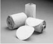
Constructed of durable aluminum oxide; works well for most wood species. The open coat feature provides a more aggressive cut than a comparable closed coat abrasive of the same grade and a special loading resistant coating makes this disc a good choice when loading is a problem. The C weight, paper backing is more durable for extended disc life and harsher sanding applications.
