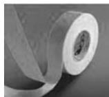
15.0 mil, white closed cell acrylic foam carrier with film liner and all purpose adhesive. High strength, handling convenience, cushioning, damping and impact resistance. UL listing 746C. 1" in width, 72 Yards per roll. P/N 09-01397 .....
