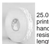
25.0 mil thick, white closed cell acrylic foam carrier with printed paper liner and an acrylic adhesive. High strength, handling convenience, cushioning, damping and impact resistance. UL listing 746C. 1" in Width and 72 yards in length. P/N 09-01359 .....
