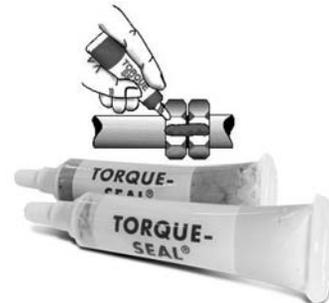
Inspection Lacquer is used in production on compression fittings, studs, nuts, parts, and assemblies after they are in proper torque or position. Widely used as "Anti-Sabotage Lacquer". Inspectors can visually detect any movement or tampering; Torque Seal becomes brittle and will crack. Excellent adhesion to all metals and to most other surfaces. Dries fast. Torque Seal is packaged in convenient 1/2 oz. poly squeeze tubes. Available in 4 high visibility.
