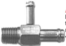
**RA1K31-4-6-4** - This 3/8" and 1/4" hose, 1/4" NPT, "T" fitting is used in most threaded ports of the flight instruments and is a FAA PMA direct replacement for the Airborne Model 1K31-4-6-4.
