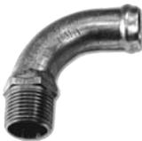
**RA1K1-6-10** - This 90° fitting with 5/8" hose and 3/8" NPT is used in most inlet threaded ports of 200 series vacuum pumps and is a FAA PMA direct replacement for the Airborne Model 1K1-6-10. This 90° fitting has superior flow and low pressure loss.
