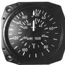
Falcon Gauge Airspeed Indicators have been one of the most chose flight instruments by kit plane builders and pilots. There are many great advantages to using these gauges: excellent slow speed characteristics; very progressive increments; a variety of ranges, light weight; short length, and affordable price. All Falcon Gauge Airspeed Indicators are housed in an aluminum case and consist of all metal parts.
