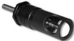
A precision tool for production countersinking. Ball thrust bearing for absolute depth control. Adjusts in .001" increments, with positive adjustment lock. Skirt accepts cutters up to 5/8" dia. Has 1/4-28 male threaded shaft for use with AT418 cutters. Can be assembled and disassembled without special tools. Split shaft and taper
