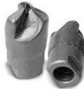
Three-straight flute replaceable pilot cutters with female thread. These cutters are designed with extra deep flute to permit numerous resharpenings and radial clearance to assure fast smooth cutting.
