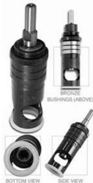
2 Models available-one with NEEDLE bearing and one with BRONZE bushings. .001" increment depth adjustment. Positive adjustment lock. 1/4" dia. shank. 9/32" shaft travel. 9/16" cutter capacity. For 1/4-28 threaded cutters. Comes with "NO-MAR" foot piece. Rated at 3,000 RPM. Made in USA.
