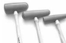
These extended depth plastic mallets allow deeper reach and a more aggressive and fuller finished shape. The UHMW polyethylene heads are lightweight, resistant to wear and non-marring. Hickory handles with full round shafts. When paired with shot bags, very creative, roughed out forms can be accomplished.
