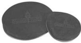
These shot bags are made out of .070/.090 thick top grain cowhide for extended life and to produce a blemish-free metal surface. These bags have suede outer or forming surface and a tanned inner surface to resist abrasive wear from the media. Convenient media filter and reinforced flap with velcro seal is provided. All bags are approximately 1.5" to 2" thick when filled. Can be filled with buckshot or silica sand (not included) found at most sporting good stores.
