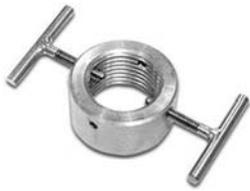
Precise Gap is a simple tool to gap two-, three- or four electrode 18 mm sparkplugs. Only 2" overall - comfortably handheld. Precision made of stainless steel. "T" handle adjusters move the ground electrodes closer to the center electrode until wire feeler identifies proper gap. Adjusters have fine thread with ball tips for precise movement. Don't buy an inferior imitation at a higher price!
