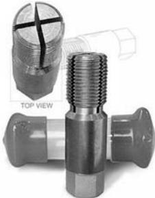
In servicing spark plugs, a common problem is carbon accumulation in the jug threads. Cleaning these threads regularly can save big money by preventing thread damage and the need to pull the jug and install thread inserts. This specially designed tool works very well to limit this problem. It provides maximum depth penetration and its unique spring action assures that there will be no enlargement of the existing thread pitch diameter.
