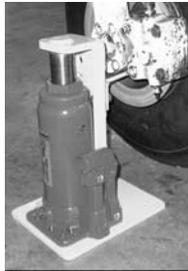
Forget expensive wing jacks for simple projects! Reach for Bogerts 6-ton Tribal Aircraft Jack! Raise each wheel independently in seconds. Service brakes or bearings, and change a tire in seconds. Adjustable lifting height, with a range of 3.5" to 11.5". Originally designed for Pipers, thus the name "Tribal Jack", it is also used on King Air, Muskateers, Debonairs, Sundowners, Mooneys and most with near vertical landing gear. Max. load is 2500 pounds.
