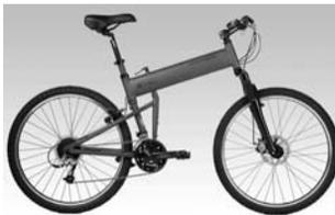
A 24-speed mountain bike which folds simply, without the use of tools. By turning one quick release lever, Paratrooper™ compacts in less than 30 seconds into a 3'x3' pack for easy portability & storage.
