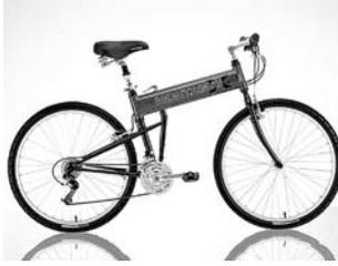
The Montague CX features 26" standard wheels, 21-speed Shimano gearing and a brushed blue aluminum / chromoly frame. Folds to 36"x 28"x 12" in under 30 seconds without use of tools, and fits easily into light aircraft, car trunk, or boats. Extra cushioned saddle and wide tires offer a smooth ride on paved road and a good grip on light off-road terrain. Excellent for cruising city streets or boardwalks.
